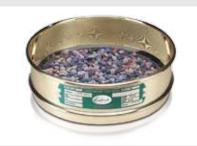
A feature of the 3D sieving action is the rapid vertical movement imparted by the shaker. The movement is continuously helping to clear apertures and avoid them blinding.
